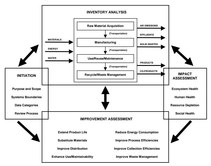
Figure 1 – LCA methodology. (Adapted from CSA, 1994b, p. 4).
