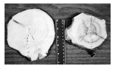
Figure 3: Discs of tree #3 from base and last measurable disc of buried stem at 64 cm.
