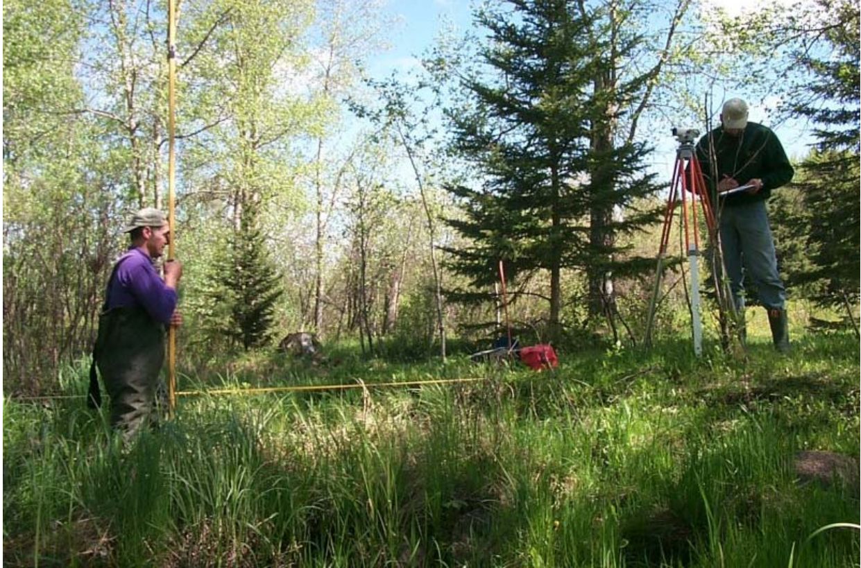
Figure 4. Surveying the cross-sectional geometry of a headwater stream.
